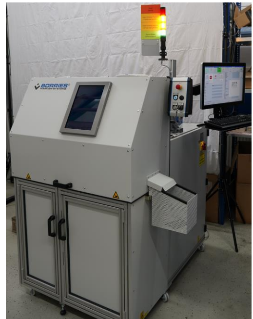
Application example: Laser cabin, front view with collection container and input PC
