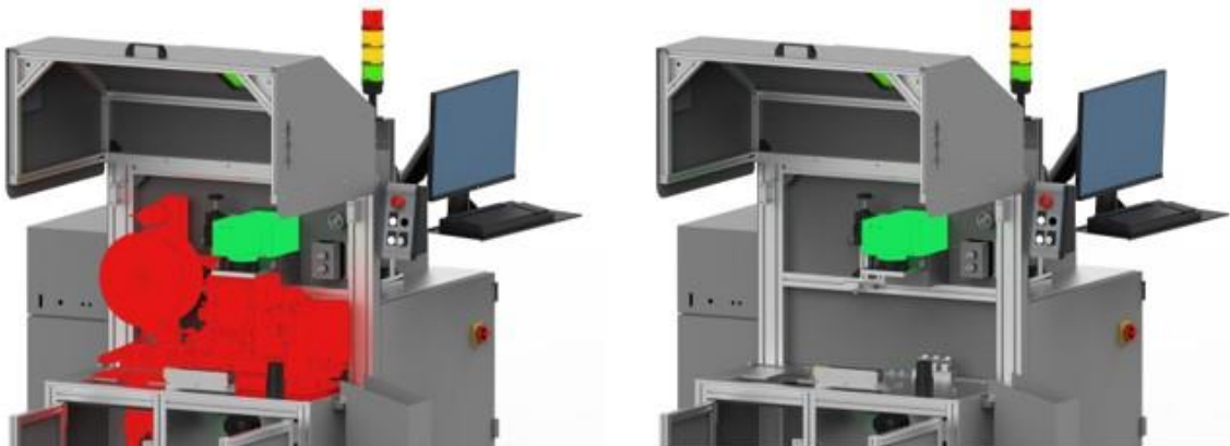
Interchangeable modules for workpiece feeding
