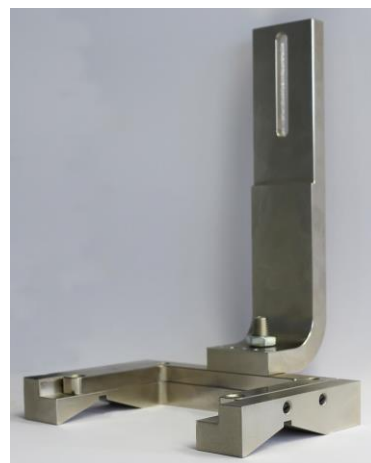
Prism holder for round workpieces are optional
